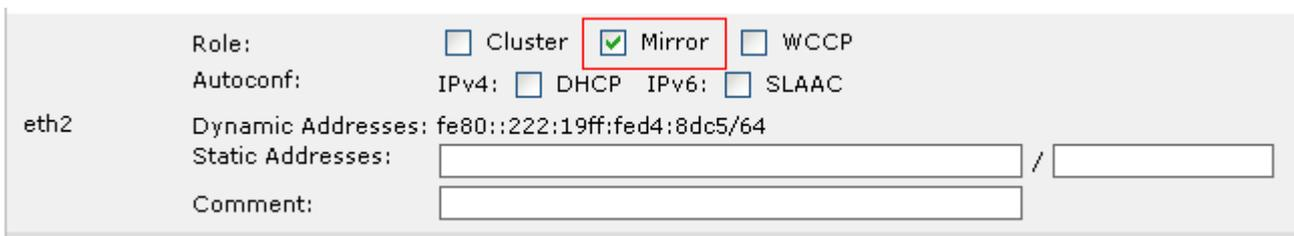
The screenshot shows the configuration page for interface 'eth2'. The 'Role' section has three checkboxes: 'Cluster' (unchecked), 'Mirror' (checked and highlighted with a red box), and 'WCCP' (unchecked). The 'Autoconf' section has two checkboxes: 'IPv4: DHCP' (unchecked) and 'IPv6: SLAAC' (unchecked). The 'Dynamic Addresses' field contains the value 'fe80::222:19ff:fed4:8dc5/64'. The 'Static Addresses' field is empty. The 'Comment' field is also empty.
