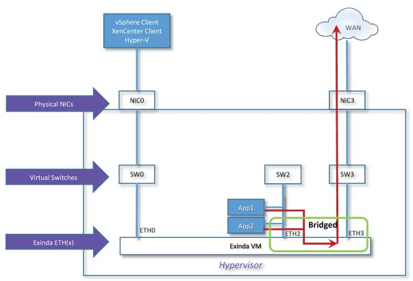
Screenshot 36: Use-case for Inline deployment with an isolated virtual LAN and virtual applications
