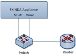
Screenshot 22: Topology diagram showing how to cable MGMT and Mirror ports for Mirror/SPAN port monitoring.
