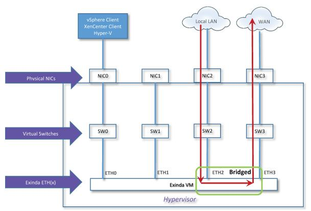
Screenshot 34: Use-case for Inline deployment with externally attached LAN
