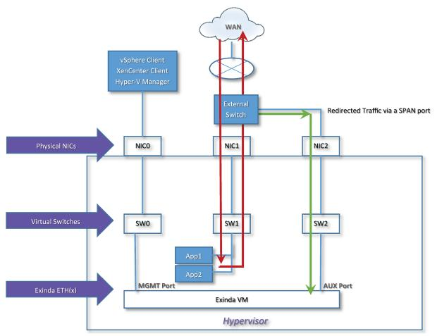
Screenshot 39: Use-case for Port mirroring/SPAN port Configuration
